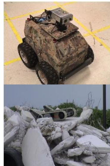
Fig. 3. A man-portable general purpose field robot (top), and a MOUT field robot exploring a rubble pile (bottom), both from manufacturer Field Y.
